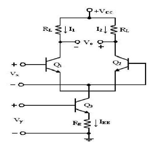
The variable transconductance technique makes use of the dependence characteristic of the transistor transconductance parameter on the emitter current bias applied. A simple differential circuit arrangement depicting the principle is shown in figure.
