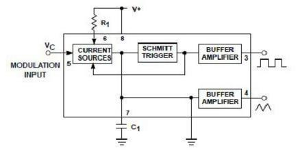
The VCO oscillates at an angular frequency,  $\omega$ out. Its frequency is set to a nominal  $\omega$ 0 when the control voltage is zero. Frequency is assumed to be linearly proportional to the control voltage with a gain coefficient KO or KVCO (rad/s/v).  $\omega out = \omega 0 + KOV cont$
