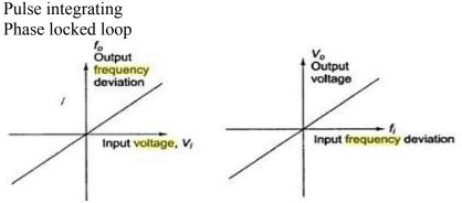
F-V convertor produces an output voltage whose amplitude is a function of input signal
