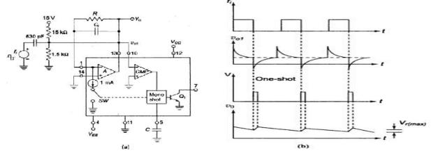
Frequency To Voltage Convertor using VFC32 (V-F) and its input output characteristics
