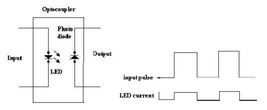
Opto couplers or Opt isolators is a combination of light source & light detector in the same package.
