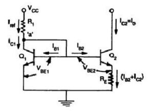
Widlar current source which is particularly suitable for low value of currents
