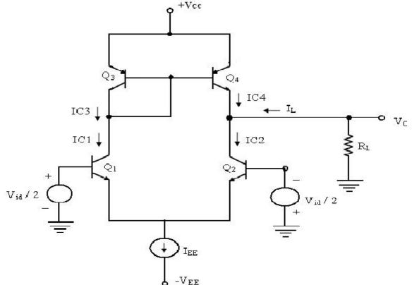
IC4 = IC3 = IC1 = gmVid/2 where IC4 = IC3 due to current mirror action. IC2 = -gmVid/2.
