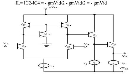
BJT Differential Amplifier with additional output stage
