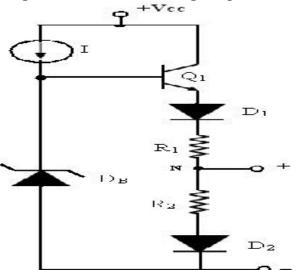
Voltage Reference circuit using Avalanche Diode Reference: (6)
