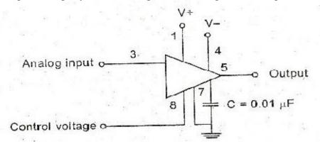
Three S/H circuits to reduce error: o series sampling,
