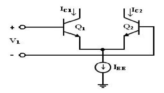
Multiplier circuit using an emitter coupled pair
