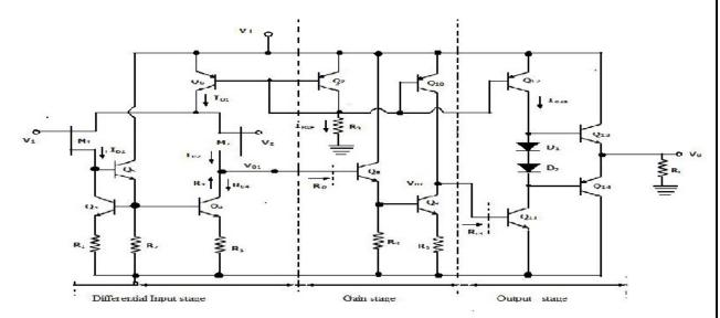
An operational amplifier generally consists of three stages, namely
