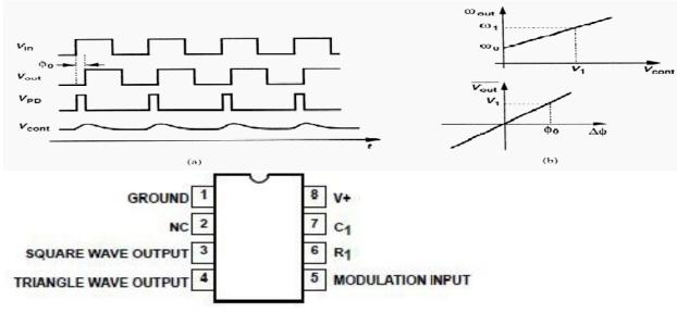
The output frequency of the VCO can be given as follows:
