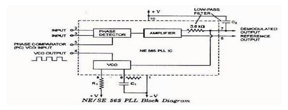
The center frequency of the PLL is determined by the free running frequency of the VCO, which is given by
