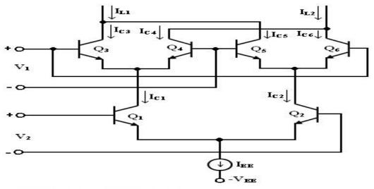
The collector current of Q3 and Q4 are given by
