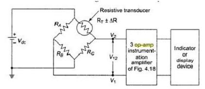
Applications of instrumentation amplifier with the transducer bridge,
