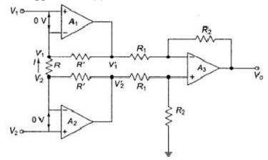
Current flowing in resistor R is I = (V1-V2)/R and it flow through R' in the direction shown, Voltage at non-inverting terminal op-amp A3 is R2V1'/(R1+R2). By superposition theorem,
