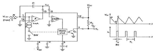
Voltage-Frequency convertor using VF32 and its input output characteristics
